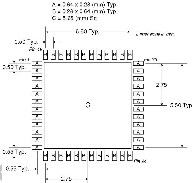
Figure 1. PCB Metal Land Pattern (Top View)
